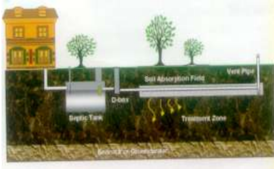
Pic. : 8 : Improper Proper Septic Tank / Flush Waste — a source of bacterial contamination of groundwater
