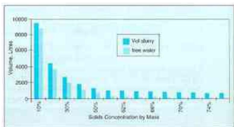
Fig. 11 Slurry and Free Water Volumes per Dry Tonne of Fly Ash
